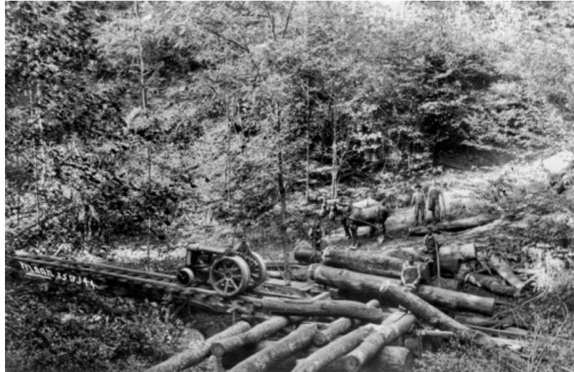
Logging operation in western North Carolina (date unknown). Horses were used to move logs to a staging area where they were picked up by a tractor on rails. North Carolina Collection, University of North Carolina
