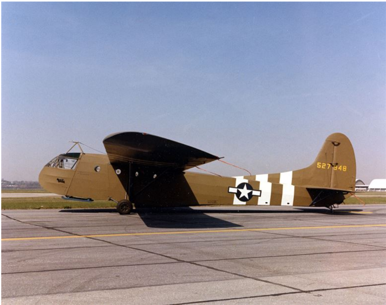
Photograph of a CG-4A World War II cargo glider, constructed of fabric-covered wood and metal. Image from the National Museum of the U.S. Air Force.
