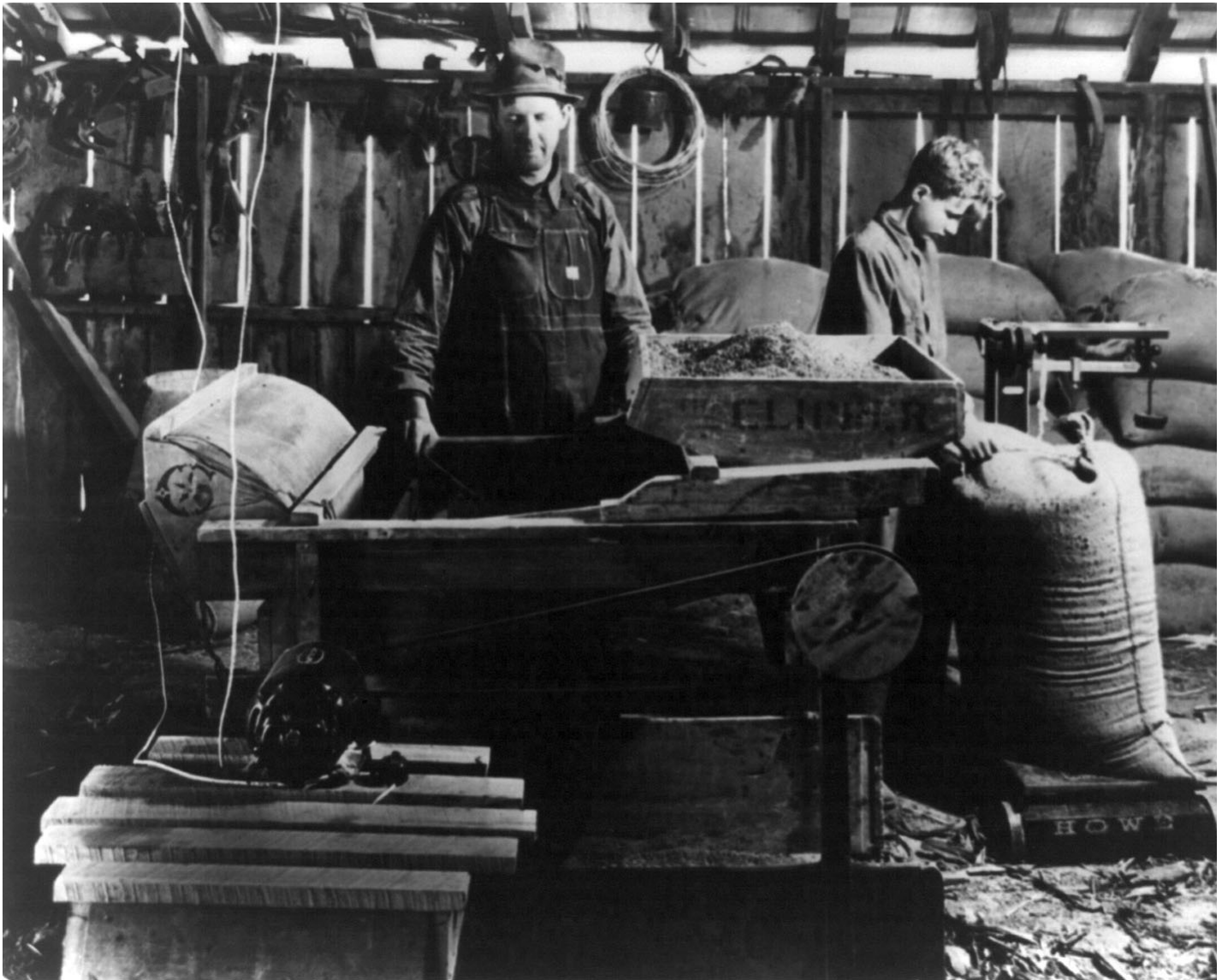
[17] Electricity also brought new technology to the farm. Many farmers built their own machinery, such as this electric-powered feed mixer.
