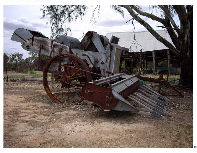
This photo is an example of a combine that added a thresher, which separated the grain from the straw at the same time, combining what had once been multiple processes.
