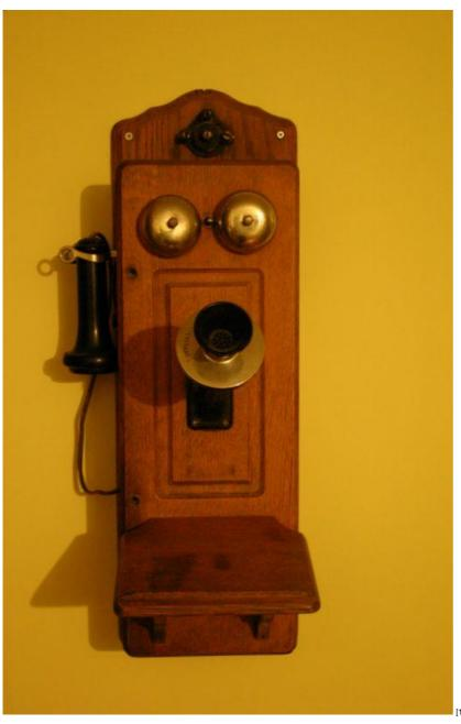
An early wall-mounted telephone, with separate earpiece and microphone.
